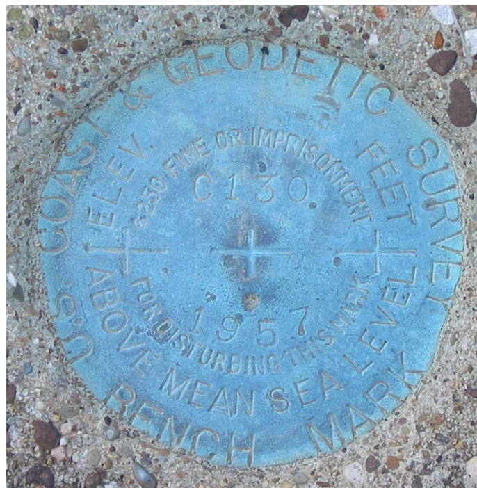
Sample US Coast & Geodic Survey Benchmark below Junior Mason's on Friendship Ridge.
